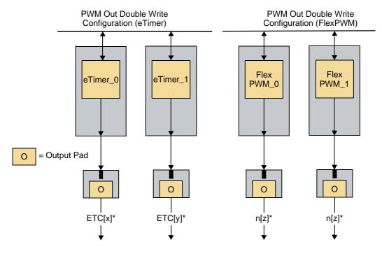
Note: n[z] represents any FlexPWM output (for example, A[z], B[z] or X[z]), but each output must be driven by different FlexPWM modules. The same consideration is valid for the eTimer; any eTimer output may be used, but each output must be driven by different eTimer module.
