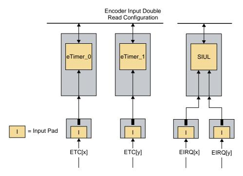
Figure 3. Double encoder read input
